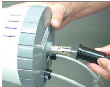
2. Slide the sleeve off the metal mounting post of the monode.
