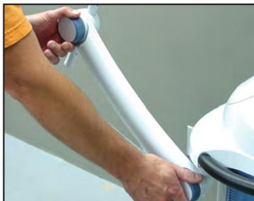
1. Loosen the front and rear handwheels and the Electrode Lock Knobs.
