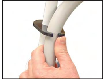
6. Fit the cord of the electrode into the cable clip on the outside of the arm.
