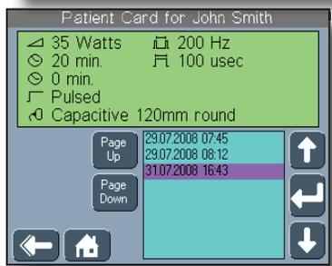
2. Press the and buttons to scroll through the treatment sessions. The treatment parameters for the highlighted treatment display at the top of the screen.
