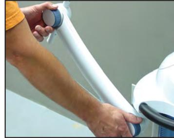
3. Tighten the front and rear handwheels and the Electrode Lock Knob to prevent movement of the arm and Monode.
