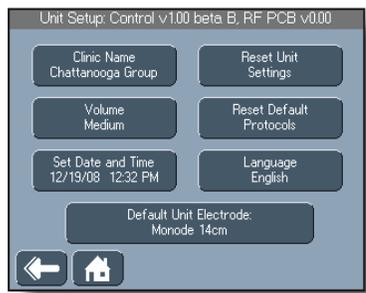
1. On the Clinical Resources screen, press the Unit Settings button. The Unit Setup screen displays.
