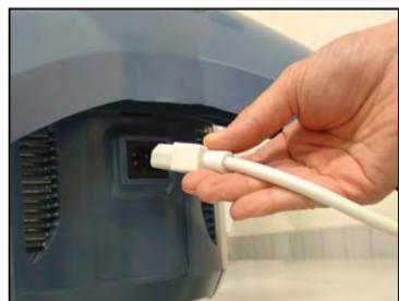
2. Connect the female end of the power supply cord into the IEC connector on the side of the unit.
