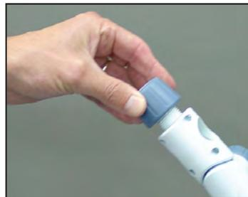
3. Loosen the Electrode Lock Knob by turning it counter clockwise.
