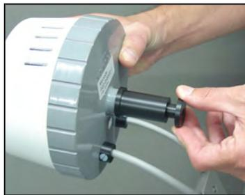
1. Remove the black, plastic retaining T nut from the sleeve by turning it counter clockwise.
