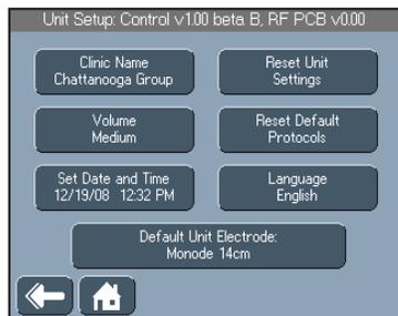
1. On the Unit Settings screen, press the Set Date and Time button. The Set Date and Time screen displays.
