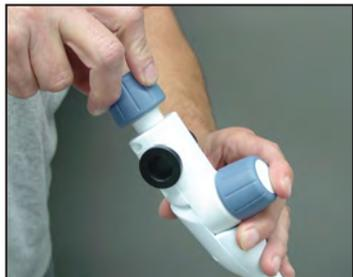
5. Tighten the Electrode Lock Knob by turning it clockwise until it is snug.
