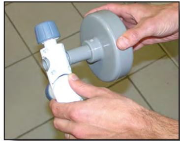
3. Push the electrode rod through the hole in the extension arm until the electrode rod is barely seen on the other side of the hole.
