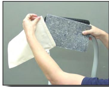
3. Slide the felt spacers and flexible rubber electrode into the linen bag.
