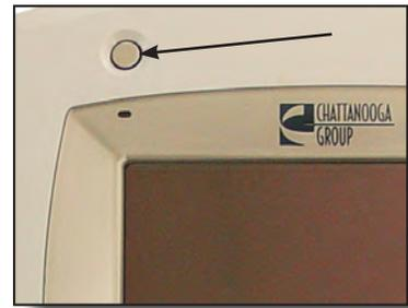
3. Press the Power On/Off button or touch the LCD. The following occurs when the Power On/Off button is pressed or the LCD is touched:
