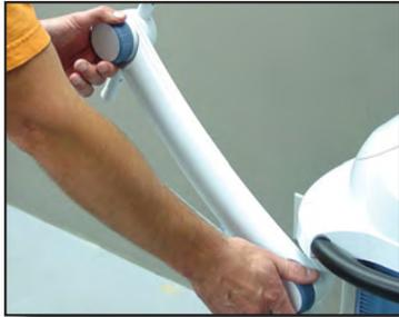
1. Loosen the front and rear handwheels and the Electrode Lock Knob of the arm that has the Inductive Applicator affixed to it.
