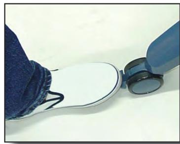
2. Depress the tabs of the castor locks to prevent the front wheels from moving.
