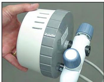
6. Push the metal mounting post of the monode completely through the sleeve.
