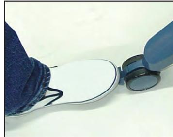
4. Depress the tabs of the castor locks to prevent the front wheels from moving.
