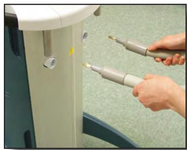
1. Plug the connectors of the flexible rubber electrodes into the output socket on the rear panel.
