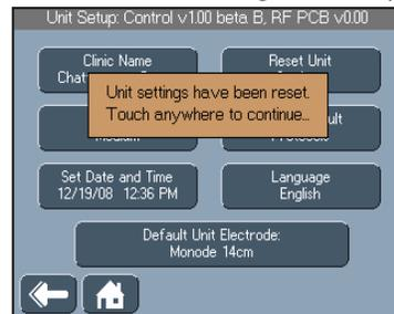
1. On the Unit Settings screen, press the Reset Unit Settings button. The reset message displays.
