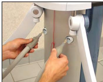
7. Plug the connector of the electrode cable into the output socket on the rear panel.
