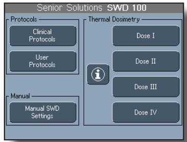
1. On the Home screen press the appropriate dose button. The Treatment screen displays with the parameters of the selected dose.
