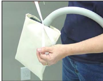
5. Tie the straps together on the linen bag to secure the flexible rubber electrodes.
