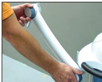
4. Tighten the front and rear handwheels and retaining sleeves to prevent movement of the arms and electrodes.
