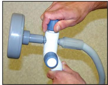
4. Tighten the Electrode Lock Knob by turning it clockwise.
