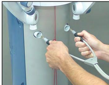
8. Plug the connectors of the monode cable into the output sockets on the rear panel.
